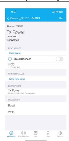
NOTICE: Measured Power which indicates RSSI@1m of iBeacon protocol is not used, the position is used to store the battery SOC, the range is from 1 to 100.
